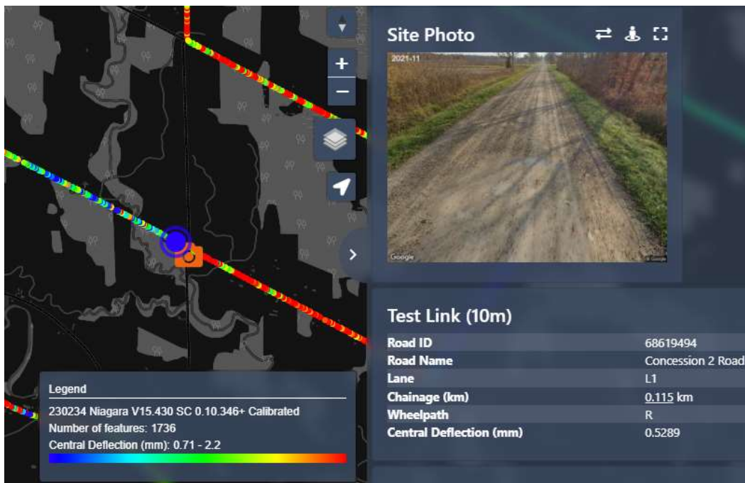
Figure 9. Example of High Deflection on a Gravel Surface.
