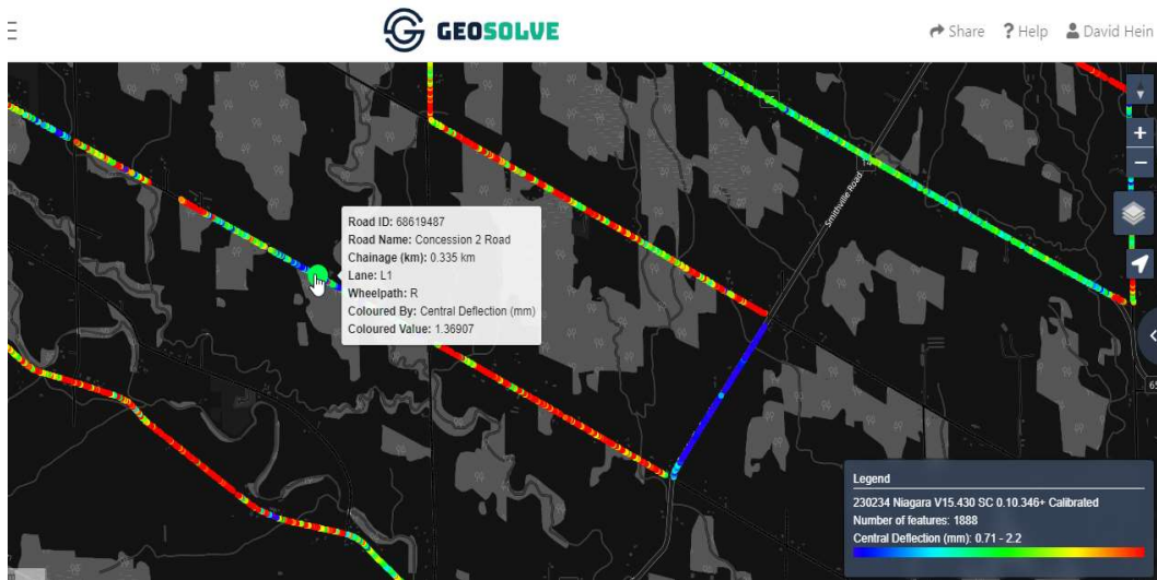
Figure 9. Example of High Deflection on a Gravel Surface.
